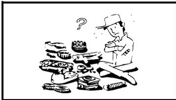
3. When disassembling the snowmobile, keep mated parts together. This includes gears, cylinders, pistons, and other parts that have been "mated" through normal wear. Mated parts must be reused or replaced as an assembly.
